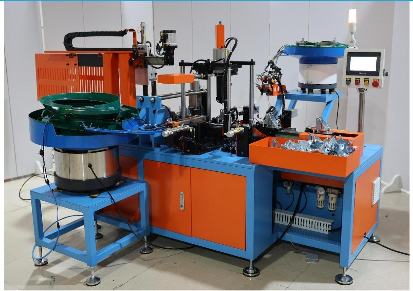
This machine is mainly for installing the brake pads of the casters
